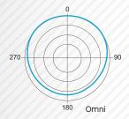
The Omni-Directional Opolar pattern picks up sound equally from all sides of the microphone. This is best used for recording in environments with excellent acoustics, as the omni-directional pickup excels at picking up ambient noise. The omni-directional polar pattern is less sensitive to "plosives", handling noise and the proximity effect.
