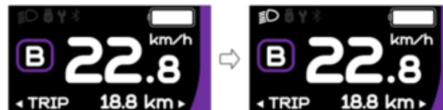
Headlight switch interface
