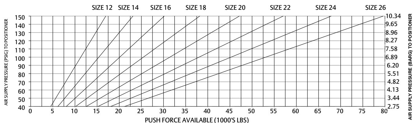
Figure A. Fisher 685 Piston Actuator Force when used with DVC6200 Digital Valve Controller
