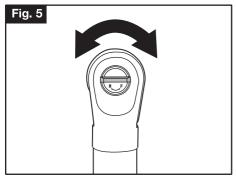
For forward (clockwise) rotation, rotate the forward/reverse toggle counterclockwise. Check the direction of rotation before use.
