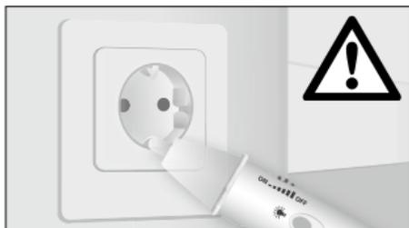
If voltage is present, the detector tip lights up and a signal sounds.
