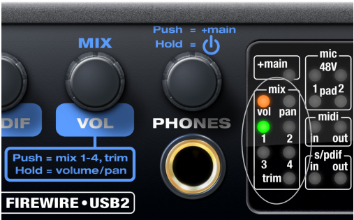
Figure 6-4: The Mix LEDs indicate which mix you are controlling with the front panel.
