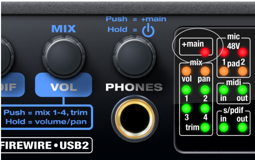
Figure 6-2: When the red “+main” LED is on, the PHONES knob controls both the headphone out and the main outs.
