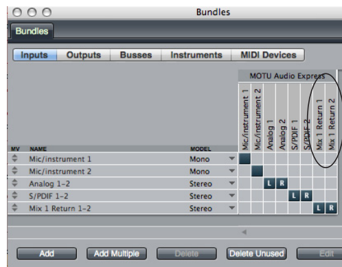
Figure 7-2: The Mix1 stereo return from the Audio Express in Digital Performer's Bundles window can be used to feed the Audio Express output back into DP.
