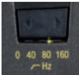
Figure 3: Bass Cut Filter
