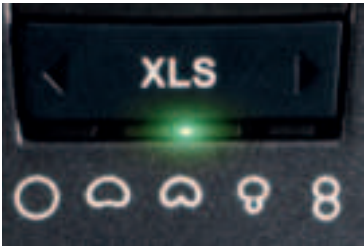
Figure 1: Polar pattern selector
