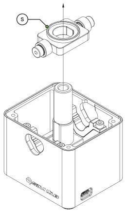
If you have trouble re installing the roller platform onto the main pivot, maybe rotate it 180 degrees. This is normal, the system is designed to have as little play as possible to work and feel as intended. Please make sure, the black nylon part is pointing upwards when installed. This is the seat (S) for the spring.
