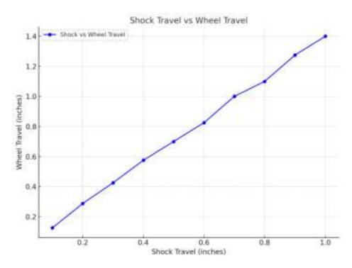
Practically, you can also plot a graph for your own setup using this exact calculation and understand how motion ratio will affect your wheel rate and will ultimately affect your car handling.
