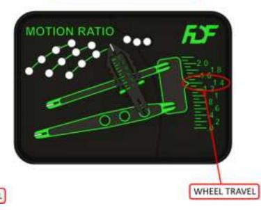
• As we can see, during the 1 inch of shock compression, Wheel has travel from 0 to 1.4 Inch. Now, lets calculate motion ratio using formula from back of the plate,
