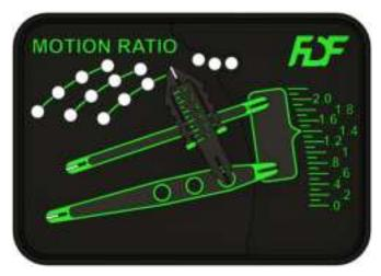
• Here, the featured Motion Ratio Display is a hands-on learning tool designed to explain the basics of Motion Ratio and Wheel Rate. Motion Ratio is critical in suspension geometry, especially with customizable suspensions. With this innovative FDF Display, understand how motion ratio can be calculated and what variables need to be adjusted in a real-world setup.
