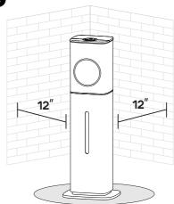
Place on a flat surface 12+ inches from walls. Use a waterproof mat underneath to catch spills.
