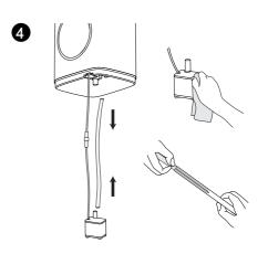
Clean the water pump with a soft brush and use a long, narrow brush to clean the silicone tube.
