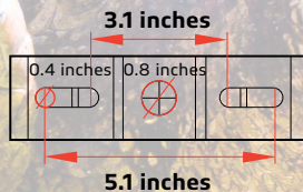
B-a. STLSTC-TRR-8W (for SUNLIKE 8W) works with 2.0 inches to 4.3 inches poles.
