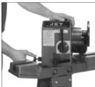
Pivoting headstock quickly turns 90° and locks to facilitate outboard turning.
