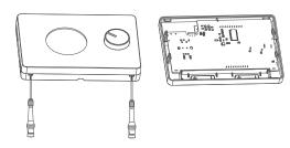
As shown in the picture above, press the screwdriver forward from the space shown, bend the tabs and separate the front cover. Insert 2 new AAA alkaline batteries in the battery housing with the correct battery direction. Replace both batteries at the same time. Then align the front part of your Room Thermostat to the back and squeeze it towards the back
