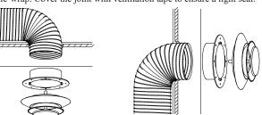
Push the pipe completely back into the structure and attach the collar to the ceiling or wall. Then attach the diffuser to its collar.
