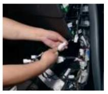
16.Plug our screen AMD's 12V male plug with original vehicel's A-pillar 12V Female plug
