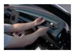
14.Use a prying tool to pry open the left and right sides of the dashboard, and take it out of the car.
