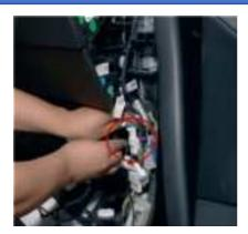
17.Plug our screen AMD's 12V female plug with original vehicel's A-pillar 12V male plug
