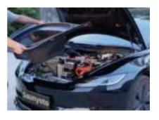
4. Remove the front trunk storage box and take it out of the vehicle. (Put the removed trim panel in the front trunk storage box for easy storage)
