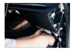
12.Remove the footwell light panel under the passenger seat and disconnect the plug
