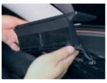
21. run the cable well, and align the air outlet of our screen with the air outlet of the original car
