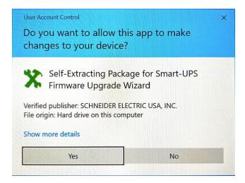
Confirm that the application is signed by Schneider Electric before proceeding.
