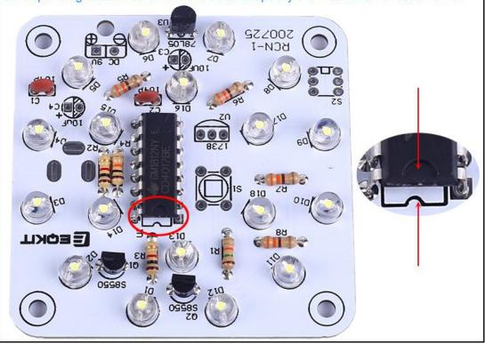
Step 10: Install 2pcs 10uF 25V Electrolytic Capacitor at C3,C4.Pay attention to distinguish between positive and negative.The Longer pin is positive pole. The longer pin is inserted into the rectangular pad.
