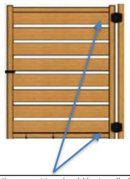
Hinges position should be installed as shown in drawing [3.5 inches from the top and bottom (B)]
