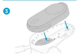
Install MEAZOR 3D by magnetically attaching the device to the Adapter. Please make sure to the device is well-coonected to the Adapter and confirm the installation is in place.
