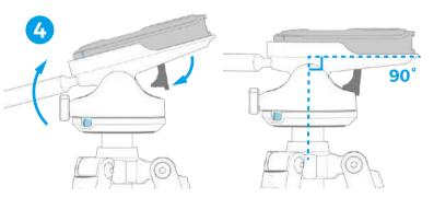
Open the vertical stand and adjust the Adapter until it is level with the ground.
