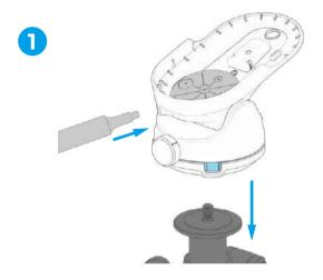
Mounting the handle and tightening the tripod
