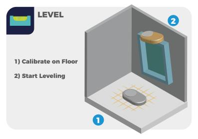
Place MEAZOR 3D on a flat surface to use the electronic level function of MEAZOR 3D. When the level is close to 0 $^{\circ}$  (<  $\pm$  1 $^{\circ}$ ), the light point turns blue.
