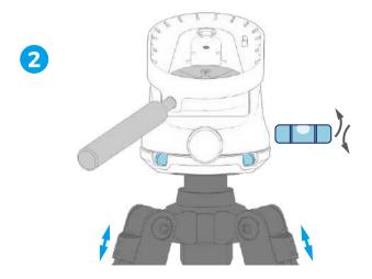
Adjust the tripod feet until the two horizontal bubble levels are centered
