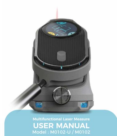
The MEAZOR 3D is a portable and multifunctional measuring device. It is composed of a 131fts (40m) laser distance module and a 4096-grade angle sensor module with high accuracy, which empowers its ability to measure straight lines, curves, and compound shapes floorplans. MEAZOR 3D is equipped with a plotting app for Android and iOS, allowing data collection, floor plan drawing, 3D display, document receiving, and
