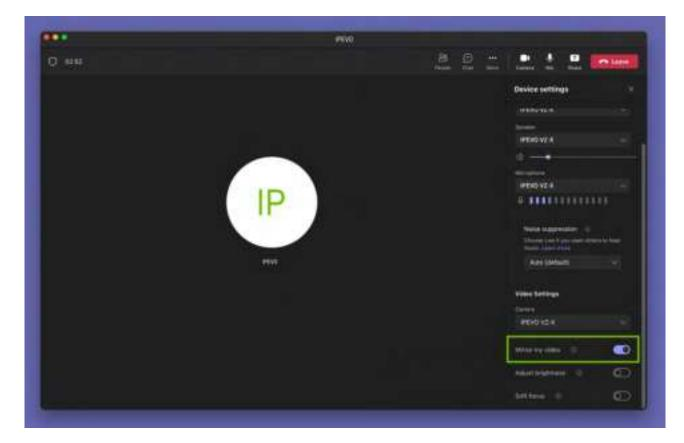
6. In the "Device settings" menu, you can also select your document camera as the microphone source. Please note that this is only possible with the document cameras, equipped with a microphone.
