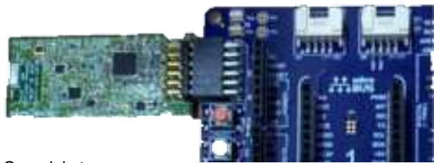
Connect Sub-G module to PMOD1 connector
