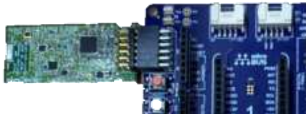
Connect Sub-G module to PMOD1 connector
