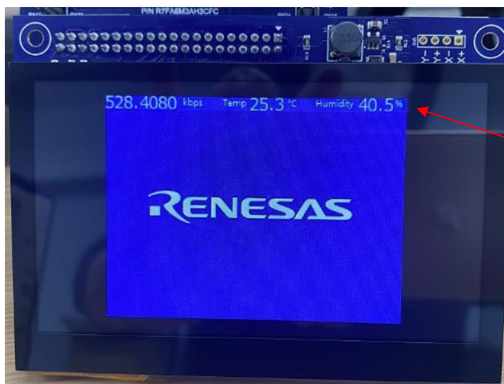
Display of throughput, temperature and humidity
