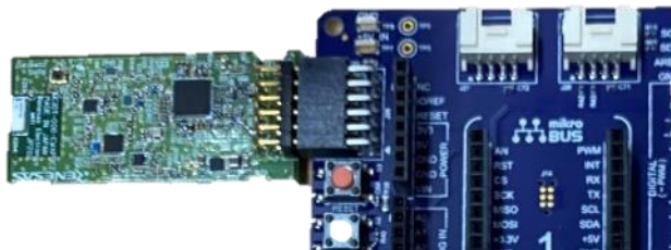
Connect Sub-G module to PMOD1 connector
