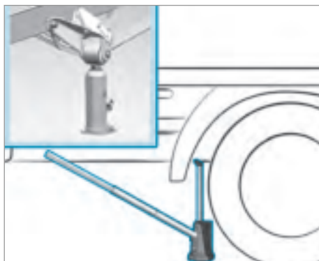
Jack support point, rear axle (example: chassis up to 3.5 t)
