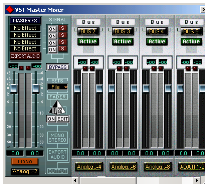
Figure 6-3: Use the output buttons at the bottom of each channel strip to assign MOTU 896 outputs to busses. You can then assign channels in the Monitor window to each bus as desired.
