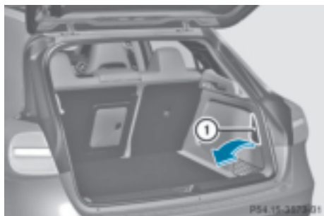
Right-hand side trim panel
