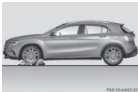
Securing the vehicle on level ground
