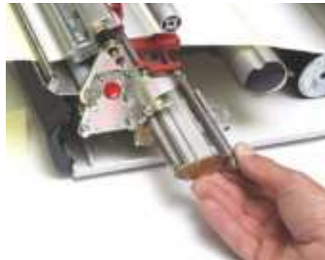
Fig. 6 Left side: pulling out the pull-out module; right side: cleaning the dispenser-feed-roller using roller cleaner.
