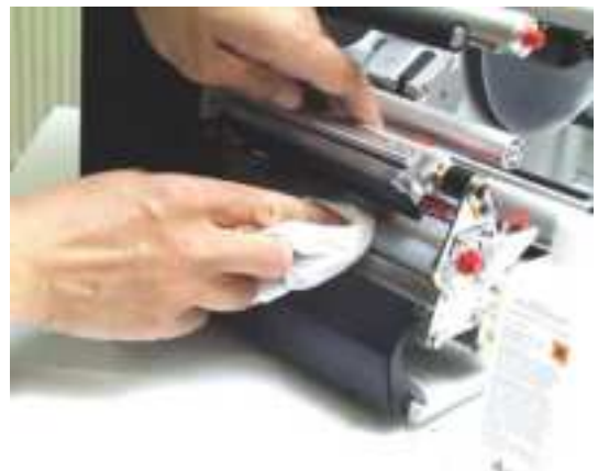
Fig. 4 Rotate the printhead upwards before cleaning it.
