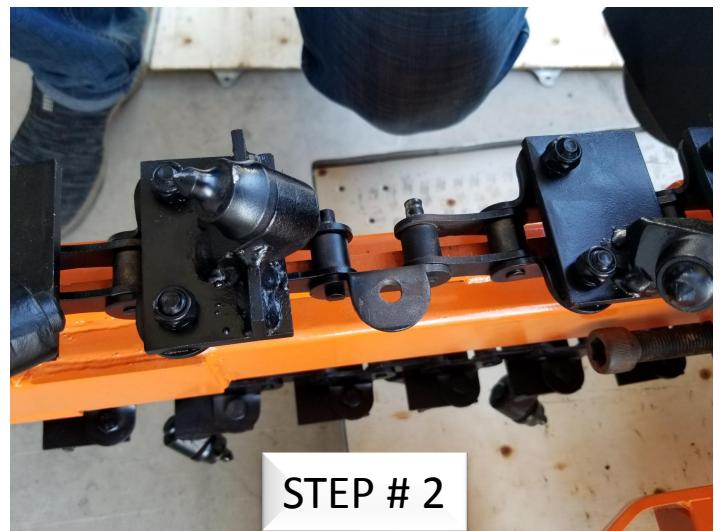
INSTALL CHAIN PLATE WITH PINS
