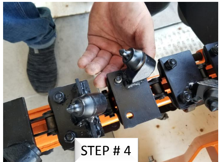
BOLT THE BLADE HOLDER ON
