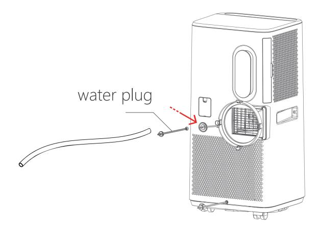
Bottom drainage port: Used when the water tank is full.
