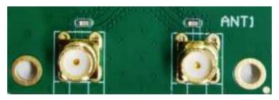
Note: The RF terminal is only connected to the antenna that needs to be used. Please do not open the software for unconnected antennas, otherwise empty space may damage the reader/writer!
