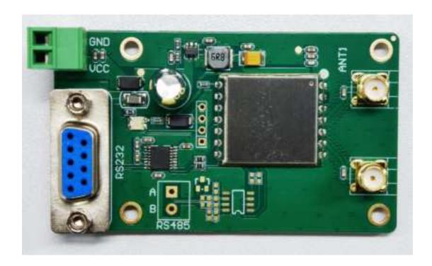
EC-RF620A-ZM is a dual-channel fixed UHF FRID reader introduced by EC-LINK, which complies with the ISO 18000-6C standard. Its operating frequency is 840MHz~960MHz. It has a compact appearance and outstanding reading and writing performance. It supports RS232 and RS485 interface data communication.
