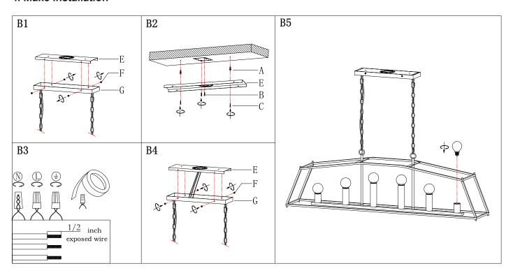
Step B1 » Unscrew canopy screws (F) from the canopy (G) and then remove the mounting plate (E).
