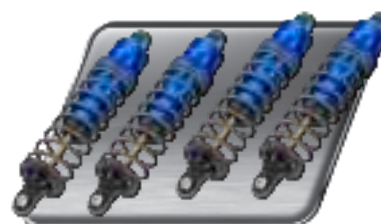
GTX Aluminum Shocks with TiN shafts
