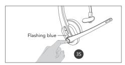
Once connected, the indicator on the Dongle will stay solid blue. The indicator on the headset will flash blue.
