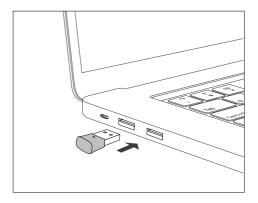
Once turned on, the indicator on the Dongle will flash quickly in blue indicating it is in pairing mode now.
