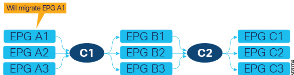
Figure 12: Prepare to begin EPG-to-ESG migration
