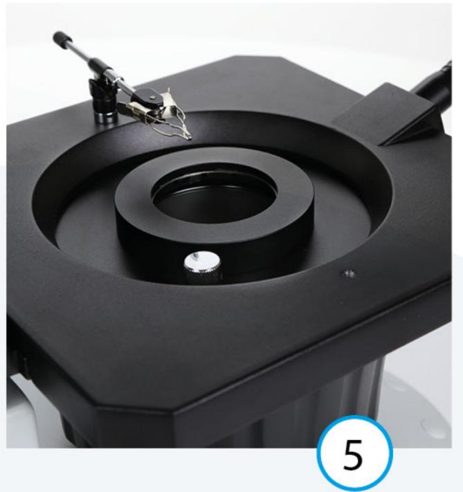
Move lever (A) to change the aperture of iris diaphragm, regulating bottom light. The aperture is ø 3mm - ø 44mm
