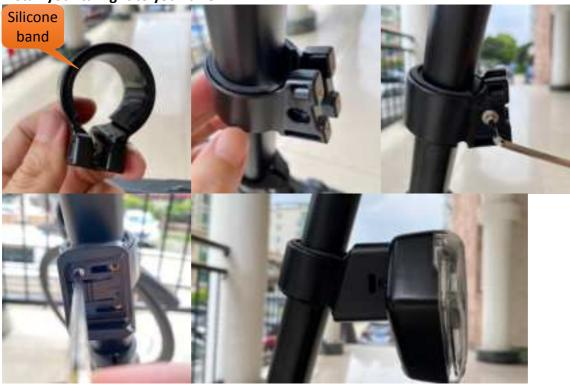
Release your taillight from mount Push the release tool into the side hole and then push taillight out of the mount.
