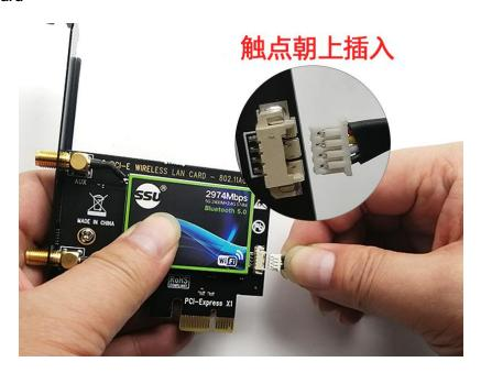
4 Align the NIC card with the gap between the chassis and the motherboard and insert it to the end
