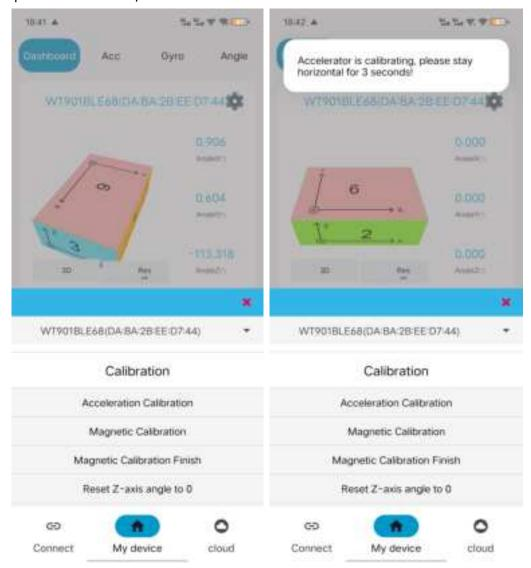
Check the result: The Z-axis angle will have less drift than before.
