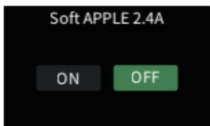
Apple devices can only charge at 5V-2.4A when detecting D+ and D- of the charger as 2.7V.
