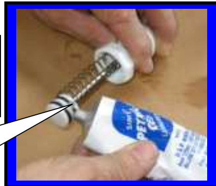
Install o-rings F0491 onto plunger
