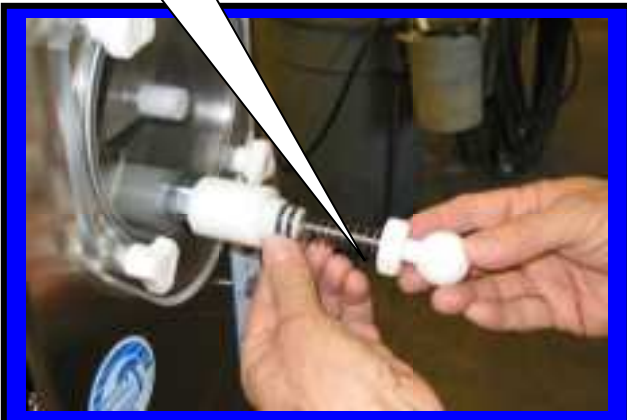
Install plunger assembly C6513P into faucet body
