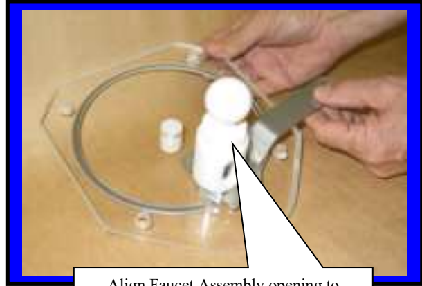
Align Faucet Assembly opening to bottom of faceplate then tighten nut
