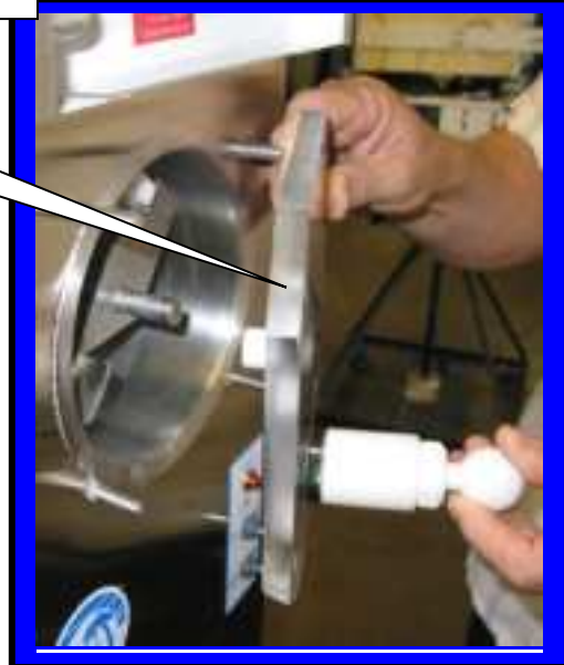
Install faceplate C6521 onto front of Machine.
