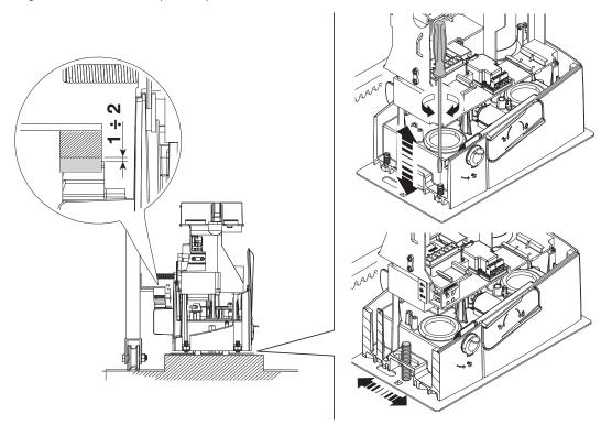
Fasten the operator to the anchoring plate using stoppers and nuts.
