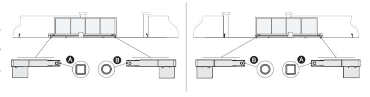
The figures below show the limit switch installed with the operator on the left.Installation of the limit switch on the right is symmetrical. Open the gate.
