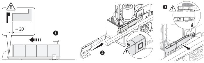
Fasten the support to the rack using the grub screws supplied.
