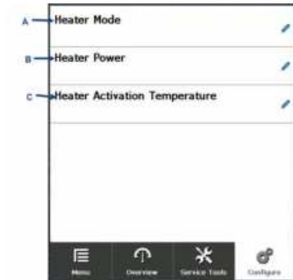
Figure 3-17: Window heater screen
