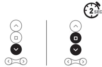
Move shade to desired bottom limit by pressing the **down arrow** repeatedly. Then press and hold **down & stop together for 2 sec** to save limit.
