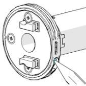
\* Internal Tubular Motor pictured. Refer to P1 Locations for specific devices Press the **P1 button** on the motor for **2 Seconds** until the motor responds as below
