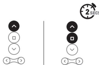
Move shade to desired top limit by pressing the **up arrow** repeatedly. Then press and hold **up & stop together for 2 sec** to save limit.
