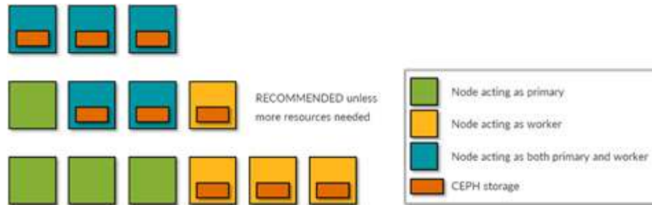
Figure 10: Multinode Redundant Setups
