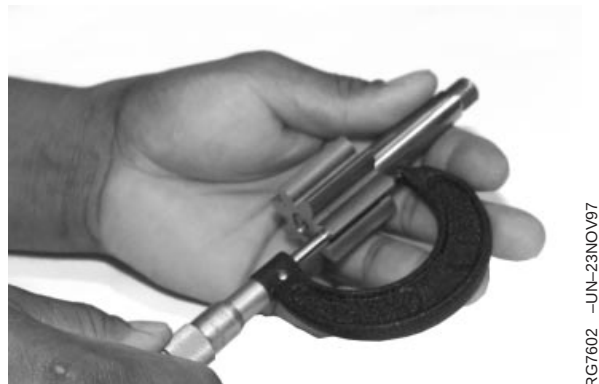
Checking Gear Thickness
