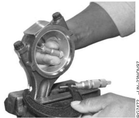
Measuring Rod Bearing ID
