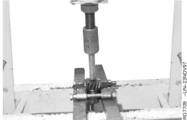
Remove Balancer Shaft Gear from Shaft
