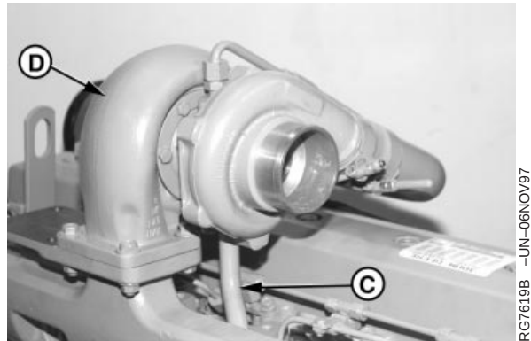
Connect Turbocharger Lines
