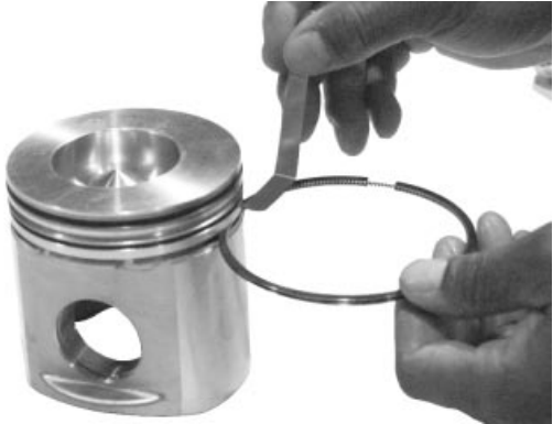
Piston Ring Groove Wear
