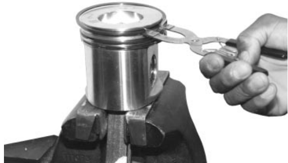
Piston Ring Removal from Piston
