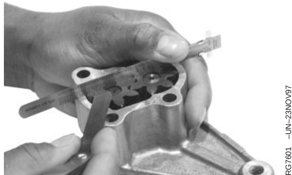
Checking Gear-to-Pump Cover Axial Clearance
