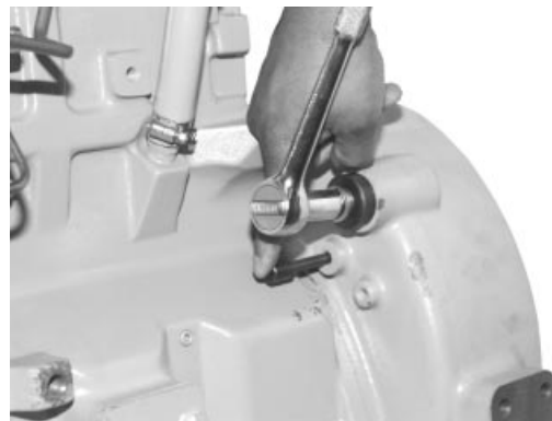
Engine Rotation Tool and Timing Pin in Place
