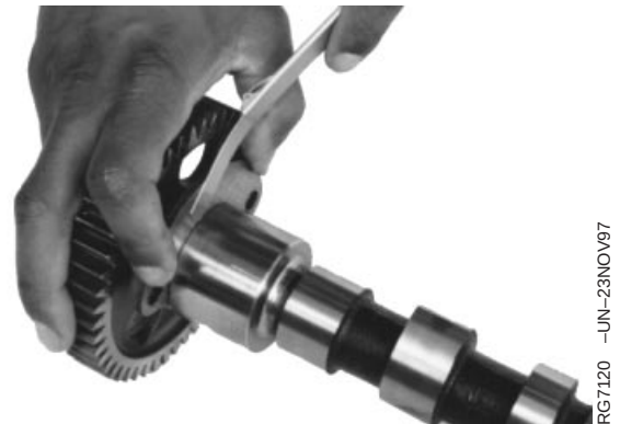
Measuring Camshaft Thrust Plate
