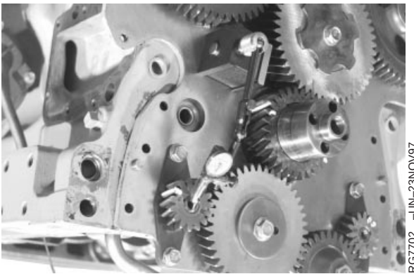
Measuring Balancer Shaft End Play—4-Cylinder
