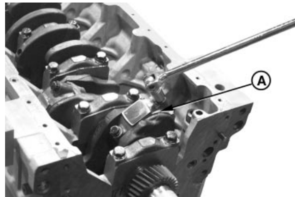
Bearing and Rod Cap Removal
