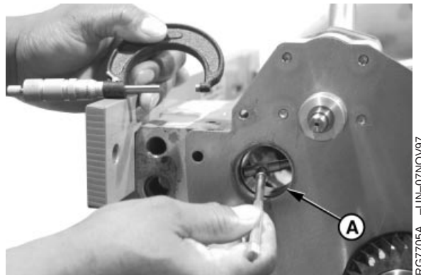
Measuring Balancer Shaft Bushing ID
