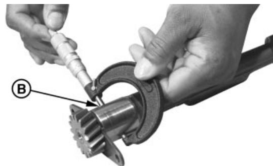
Measuring Balancer Shaft Bushing ID
