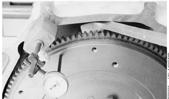
Check Crankshaft End Play w/Dial Indicator
