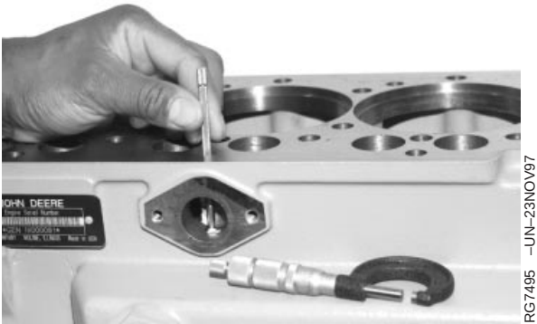
Fuel Supply Pump Push Rod Bore
