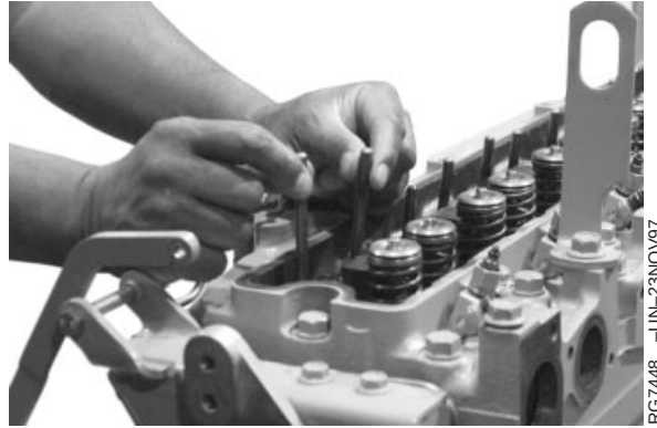
Rocker Arm Assembly Installation
