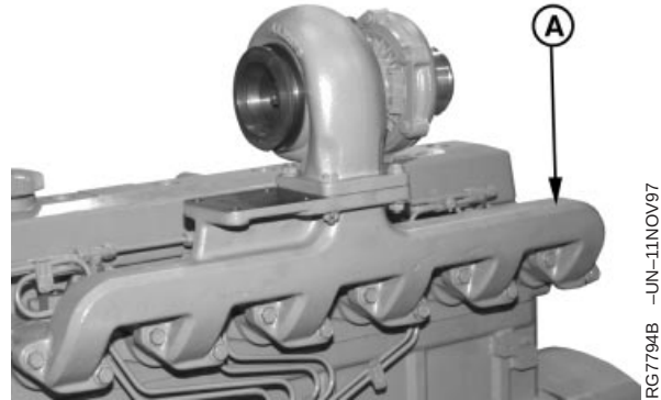
Exhaust Manifold w/Turbocharger Installed
