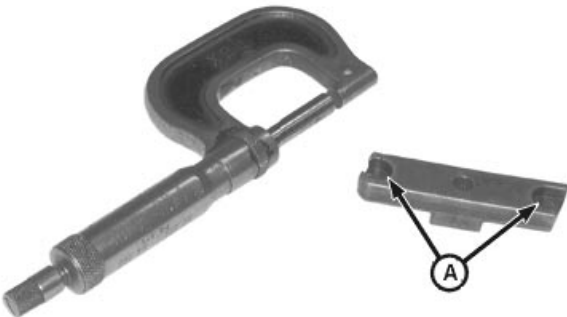
Inspect and Measure Bridges
