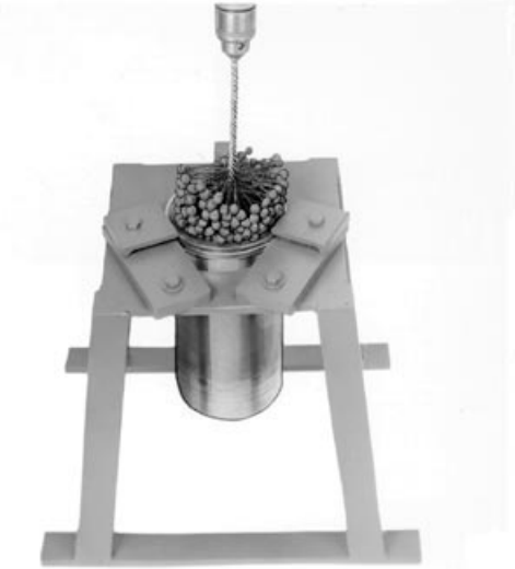
Cylinder Liner Deglazing
