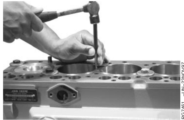
Marking Cylinder Liner Location/Position
