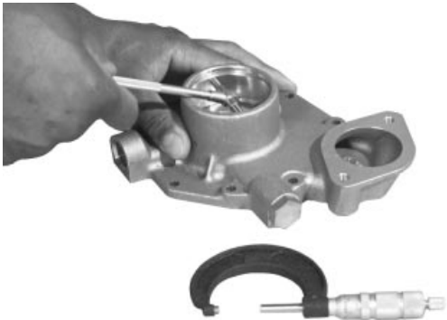
Coolant Pump Housing Weep Hole
