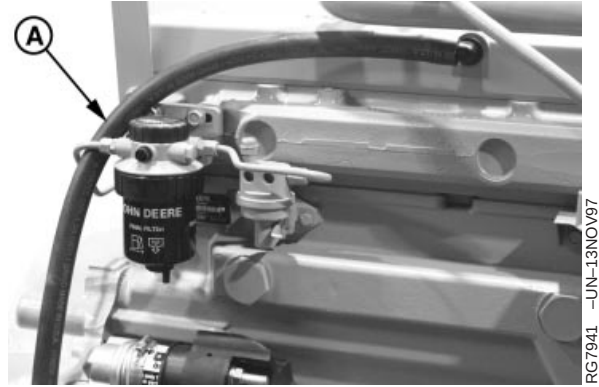
Ventilator Outlet Hose Inspection
