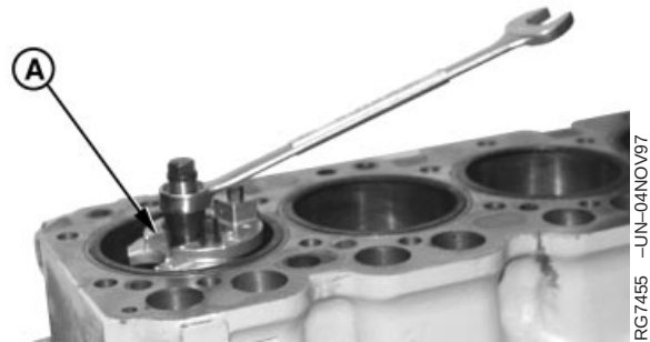
Using Ridge Reamer in Cylinder Bore
