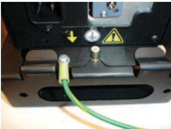
Figure 1 — Redundant Earth Ground Attachment
