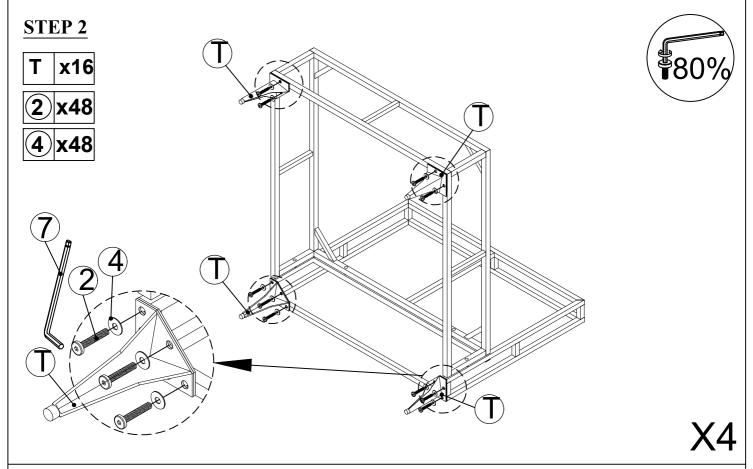
Connect the part from step 1 with Leg (T), Tighten Bolt (2) & Flat Washer (4) with Allen Key (7).
