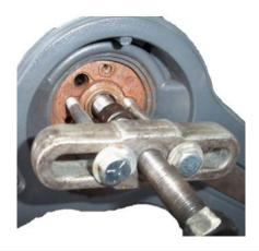
**STEP 7:** Using a marker, make reference marks on locking plate to maintain correct orientation.
