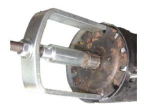
**STEP 8:** Reinstall steering wheel using marks made during removal to maintain original orientation.
