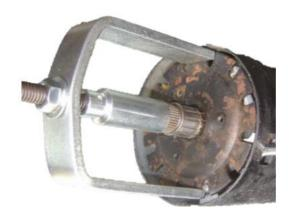
**STEP 9:** Remove snap ring while plate is compressed.
