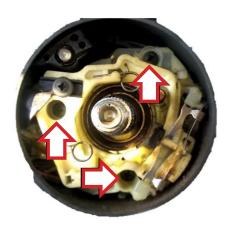
**STEP 14:** It is not necessary to completely remove switch from column. Lift turn signal switch out of way to gain access to lock cylinder release tab.
