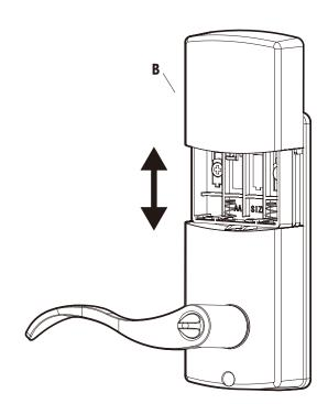
This electronic lock requires (4) High Quality AA alkaline batteries. When all 4 batteries are installed in the correct position, you should hear 2 beeps and the keypad will illuminate.
