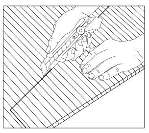
Then use a utility knife or circular saw to cut along the line.
