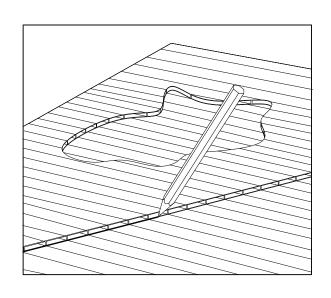
Place the original damaged polycarbonate sheets over the new polycarbonate sheets and mark along the edge with a pencil.
