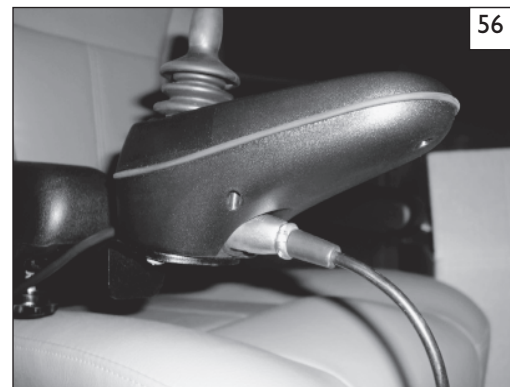
Off-board charger port located under joystick
